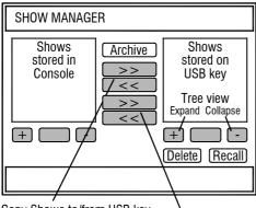
Copy Shows to/from USB key Move Shows to/from USB key
